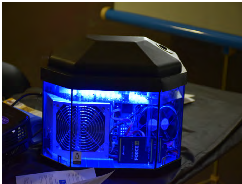
Submerged computer into a liquid coolant (Credit: Kowalski7cc)
