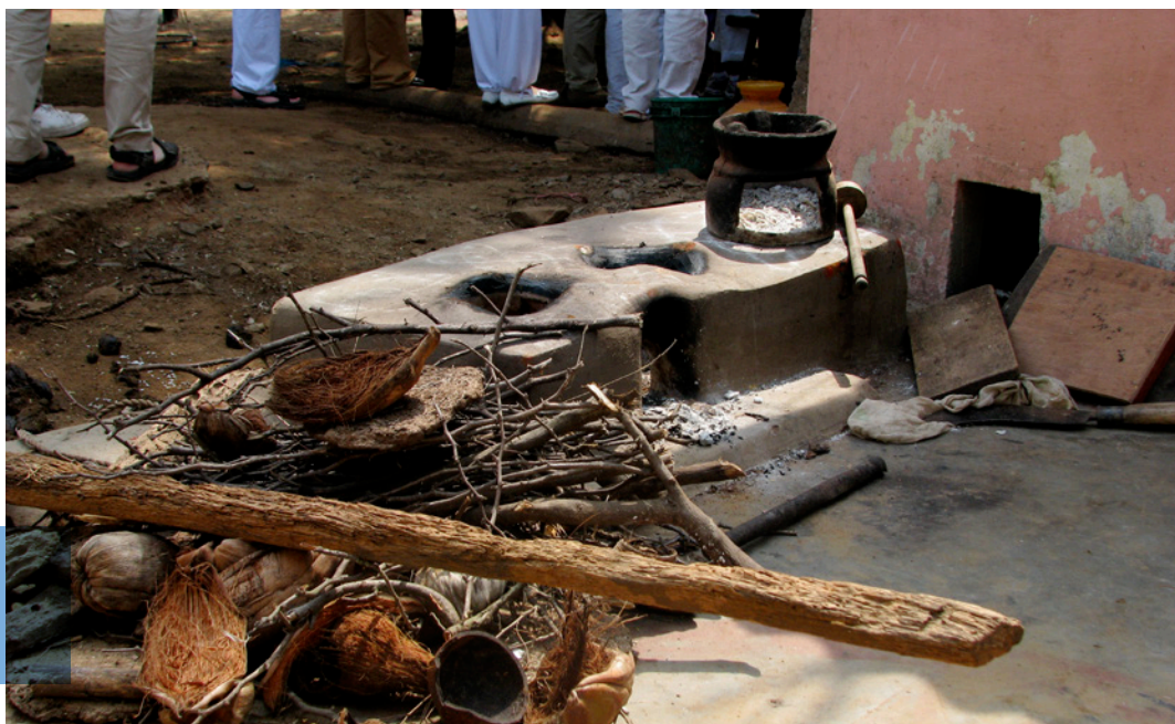
A "chulla" in Tamil Nadu, India, which is a traditional outdoor stove that burns biomass
